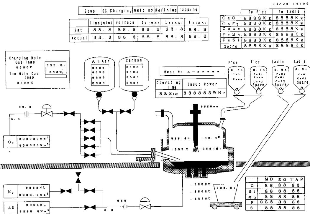
Fig. 12 Example of CRT monitor for operation
