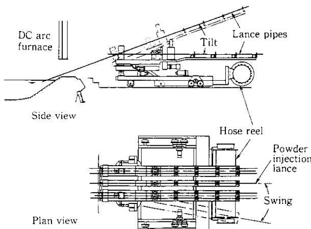
Fig. 11 Schematic diagram of oxygen blowing and powder injection device
