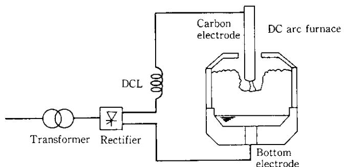
Fig. 1 Schematic diagram of DC arc furnace
