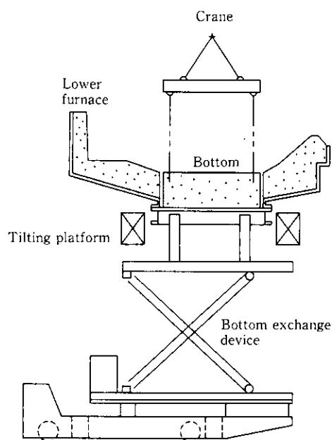
Fig. 9 Schematic diagram of bottom electrode exchange method
