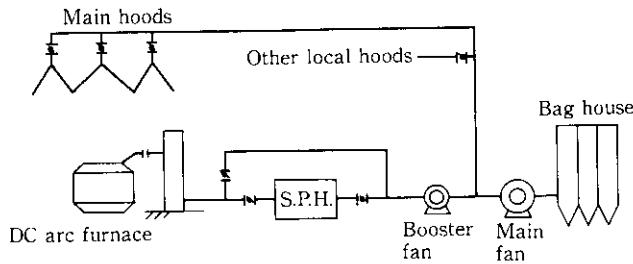
Fig. 13 Schematic diagram of dust collection equipment
