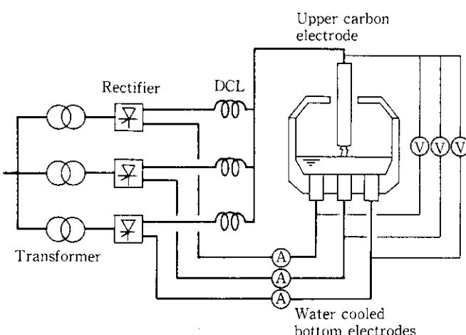
Fig. 3 Skeleton for control of arc direction
