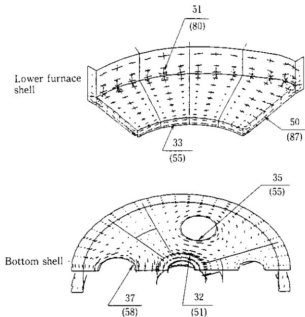
Fig. 10 Results of stress analysis of lower furnace shell and bottom shell
