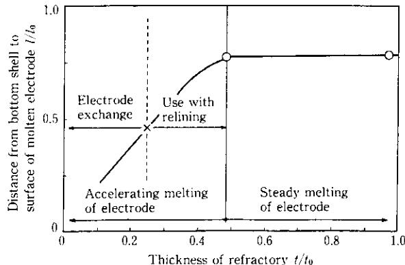
Fig. 8 Effect of refractory thickness on the amount of bottom electrode melting
