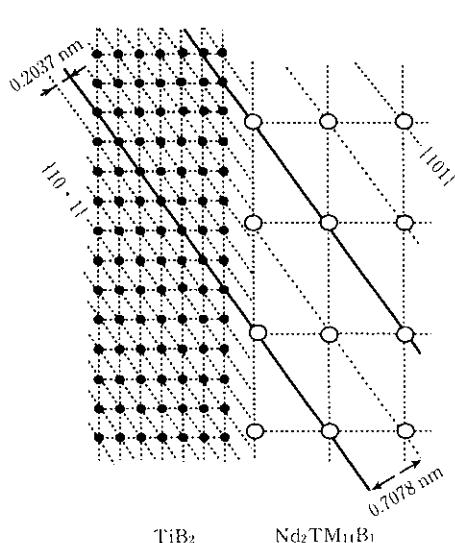
Fig. 3 The schema of the nano-sized  $\text{TiB}_2$  precipitated intragranularly in the  $\text{Nd}_2\text{TM}_{14}\text{B}_1$  phase
