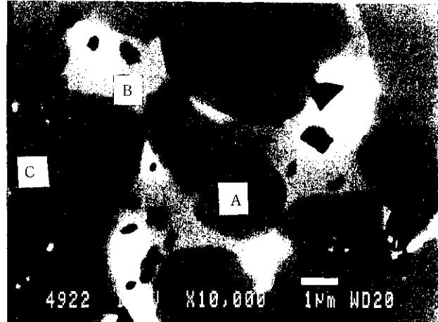
Photo 3 Backscattered electron image of the  $\text{Nd}_{15}(\text{Fe}_{0.585}\text{Co}_{0.3}\text{Ni}_{0.1}\text{Ti}_{0.015})_{77}\text{B}_8$  sintered magnet ( $\text{Nd}_2\text{TM}(=\text{Fe}, \text{Co}, \text{Ni})_{14}\text{B}_1$ , phase A;  $\alpha'\text{-Nd}$ , phase B; and  $\text{TiB}_2$ , phase C)
