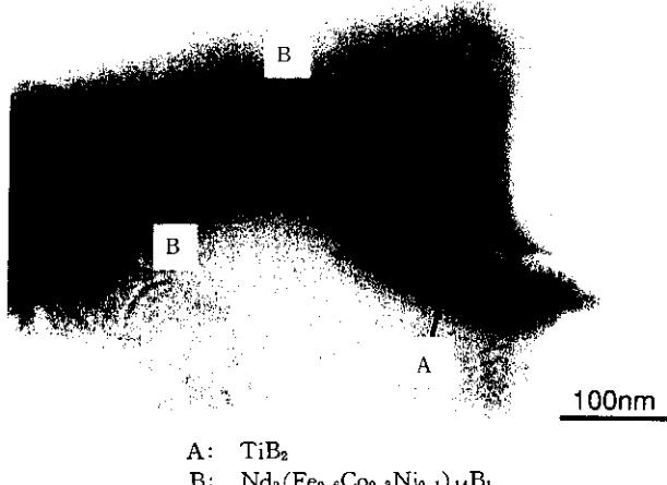
Photo 5 Transmission electron image of intragranular precipitate TiB<sub>2</sub> in the Nd<sub>15</sub>(Fe<sub>0.585</sub>Co<sub>0.3</sub>Ni<sub>0.1</sub>Ti<sub>0.015</sub>)<sub>77</sub>B<sub>8</sub> sintered magnet
