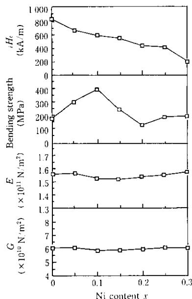
Fig. 1 Ni concentration dependence of the intrinsic coercivity  $H_c$ , bending strength, Young's modulus  $E$  and shear modulus  $G$  for  $\text{Nd}_{15}(\text{Fe}_{0.6-x}\text{Co}_{0.3}\text{Ni}_x\text{Ti}_{0.015})_{77}\text{Ba}$  sintered magnets
