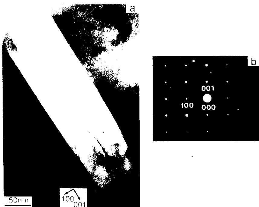
Photo 4 Transmission electron image with crystal orientation (a) and electron-diffraction pattern of intergranular precipitate  $\text{TiB}_2$  (b) in the  $\text{Nd}_{15}(\text{Fe}_{0.585}\text{Co}_{0.3}\text{Ni}_{0.1}\text{Ti}_{0.015})_{77}\text{B}_8$  sintered magnet
