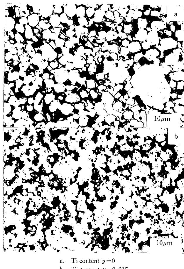
Photo 2 Micrographs of  $\text{Nd}_{15}(\text{Fe}_{0.6-y}\text{Co}_{0.3}\text{Ni}_{0.1}\text{Ti}_y)_{77}\text{B}_8$  sintered magnets
