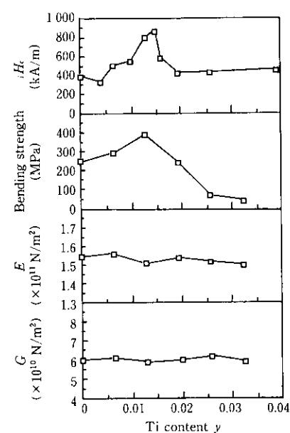
Fig. 2 Ti concentration dependence of the intrinsic coercivity  $H_c$ , bending strength, Young's modulus  $E$  and shear modulus  $G$  for  $\text{Nd}_{15}(\text{Fe}_{0.5-y}\text{Co}_{0.3}\text{Ni}_{0.1}\text{Ti}_y)_{77}\text{B}_8$  sintered magnets
