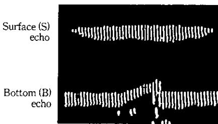
Fig. 5 An example of B scope projection (Scan mode: 8 bit group, 1 bit shift)
