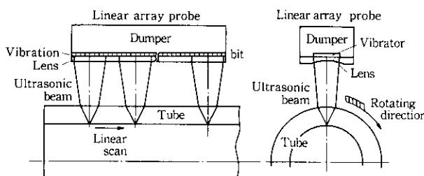
Fig. 4 Testing principle by linear array probe
