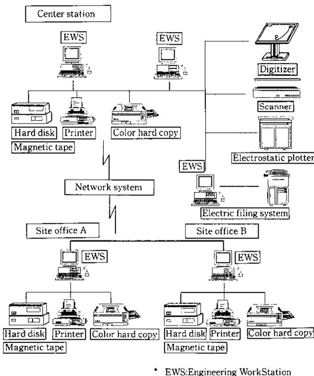
Fig. 2 Configuration of hardware
