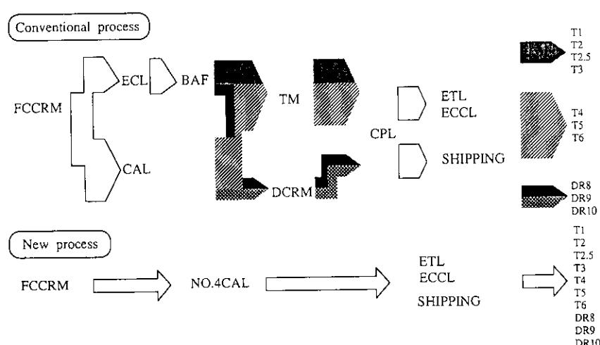
Fig. 9 Comparison of conventional process and new No. 4 CAL process for producing tinplate
