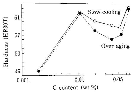
Fig. 1 Effects of carbon content and heat cycles on hardness of tinplate
