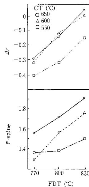
Fig. 5 Effects of hot rolling conditions, CT and FDT, on  $\tau$ -values and their planar anisotropy  $\Delta r$  on commercially produced Nb-added extra low-carbon tinplate
