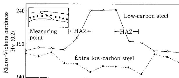
Fig. 10 Effect of steel type on micro-Vickers hardness distribution in welded seam
