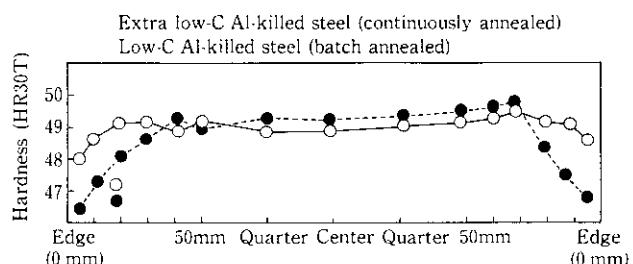
Fig. 6 Distributions of hardness in transverse direction of two kinds of tinplates
