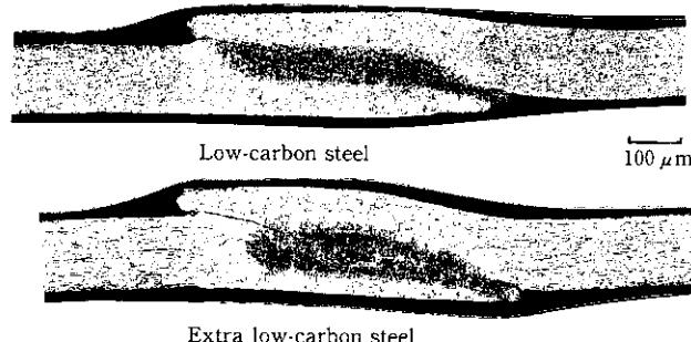
Photo 1 Effect of steel type on cross section microstructure in welded seam
