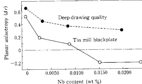
Fig. 2 Effect of Nb on planar anisotropy of r-value ( $\Delta r$ ) in cold rolled steels of tin mill blackplate and deep-drawing quality
