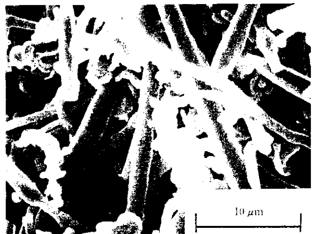
Photo 2 Scanning electron micrograph of thick SiC whisker with diameter of 1.85 \mu m
