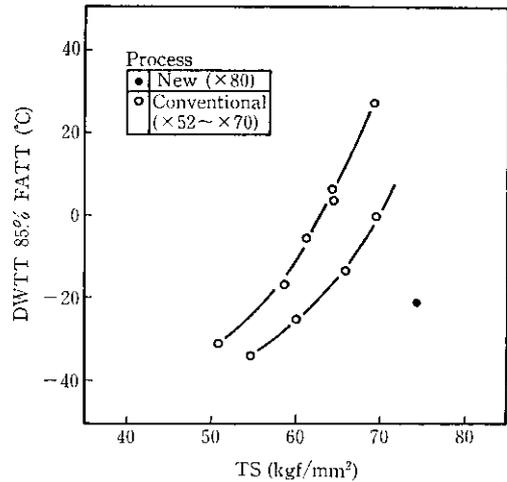
Fig. 11 Effect of new process on TS-85% FATT relation of pipes (API 5L X52~X80,  $t=0.500''\sim 0.625''$ , test direction C)
