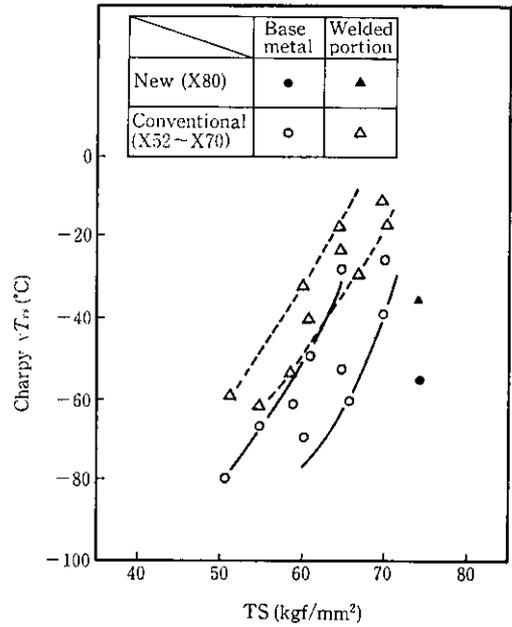
Fig. 10 Effect of new process on TS- $vT_{rs}$  relation of pipes (API 5L X52~X80,  $t=0.500''\sim 0.625''$ , test direction C, specimen size 10 mm × 10 mm)
