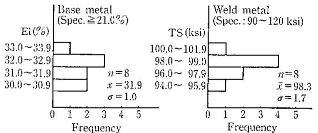
Fig. 7 Tensile properties of API 5L X80 (26"φ×0.574"t)
