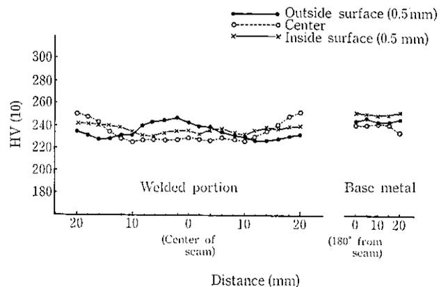
Fig. 12 Hardness properties of API 5L X80 (26''φ × 0.574''t)
