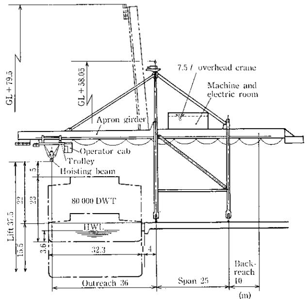
Fig. 3 General arrangement of loader
