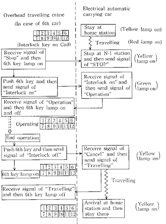
Fig. 11 Flow of controlling automatic carrying car
