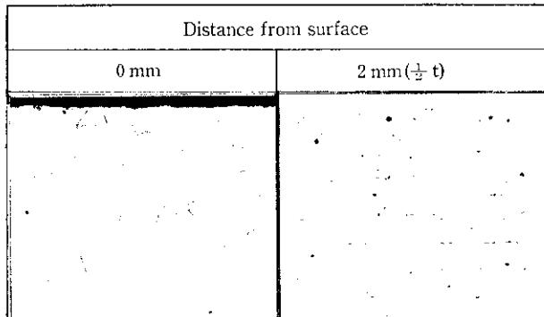
Photo 1 Microstructures of SUS 304 floor plate after electro-lytic etching in 10% oxalic acid solution
