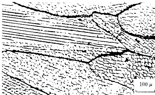
Photo 2 Micro hot cracks in welded cross bead
