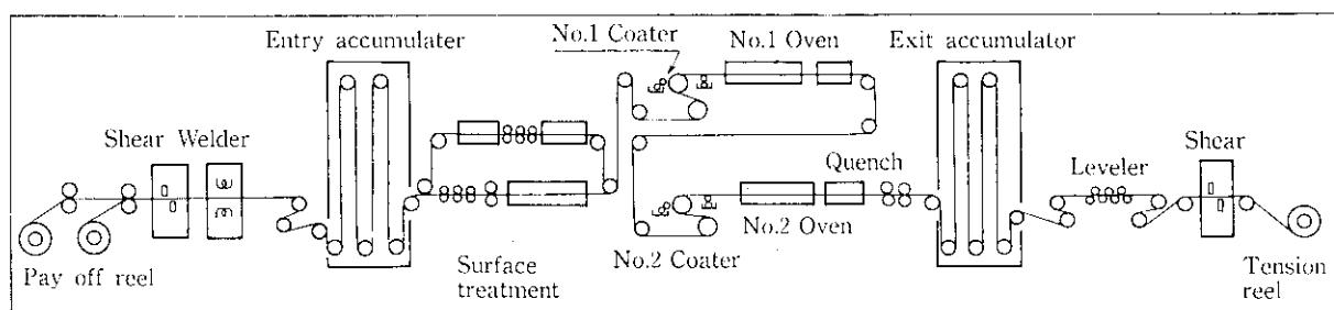
Fig. 2 Schematic diagram of coil coating line
