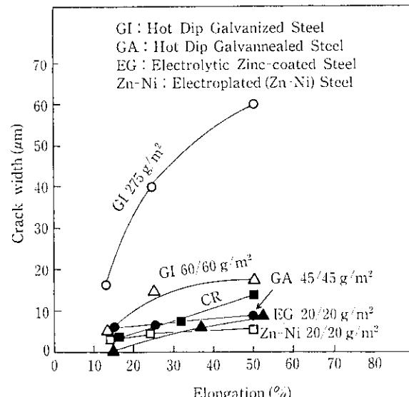
Fig. 5 Relation between elongation and crack width of surface treated steels
