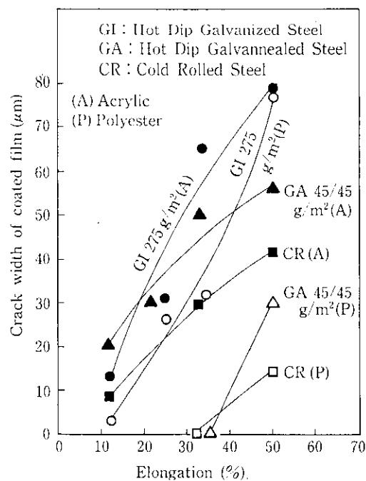
Fig. 6 Relation between elongation and crack width of coated film on surface treated steels
