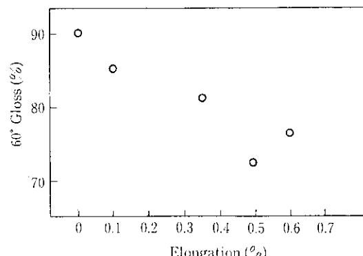
Fig. 4 Relation between gloss and elongation by tension leveler in CCL
