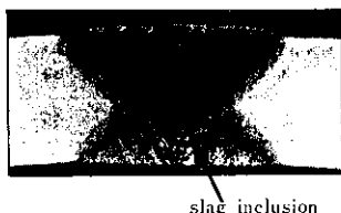
Photo. 2 Typical view of slag inclusion in external weld bead
