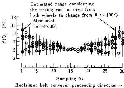
Fig. 5 Comparison of estimated and analyzed content of SiO<sub>2</sub> in ore bed quality monitoring system
