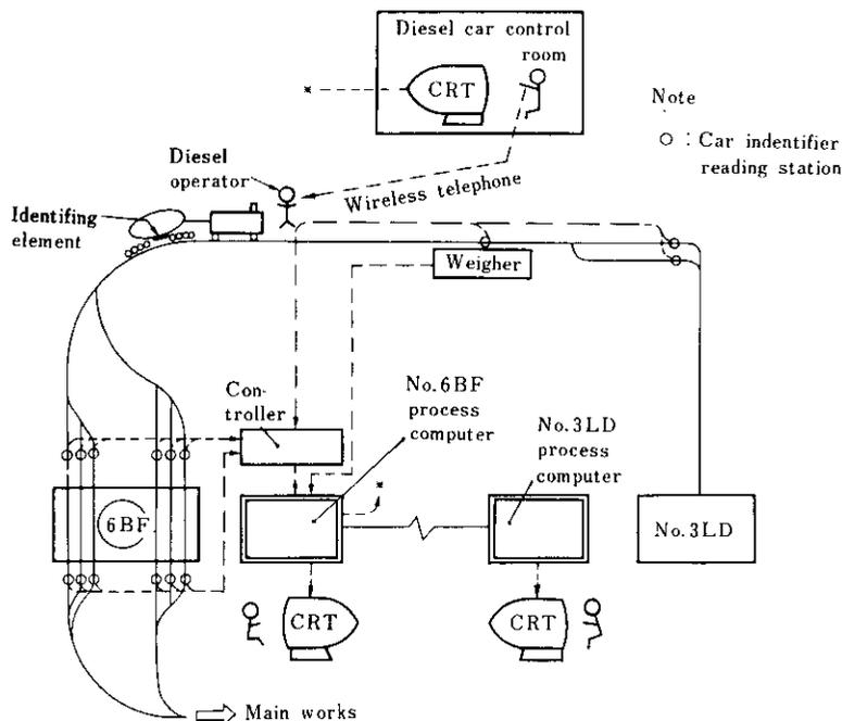
Fig. 18 Torpedo car tracking system at Chiba Works
