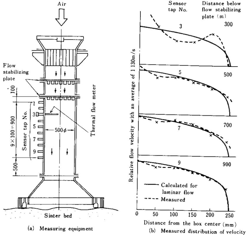
Fig. 4 Gas flow measurement on a sintering bed
