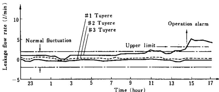
Fig. 16 An example of tuyere leakage detection system
