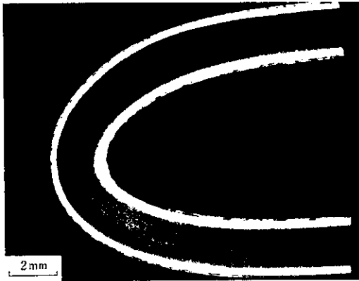
Photo. 3 Results of bend test after quenching and tempering of RFX 50
