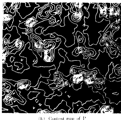
Photo. 5 Dendritic structure and content map of P of uni directionally solidified specimen (Fe-C-Zr-S-0.1%P alloy, with solidification rate of 200\text{mm}\cdot\text{h}^{-1} )
