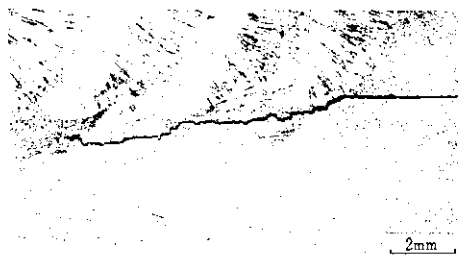
Photo. 1 Lamellar tearing in Cranfield test
