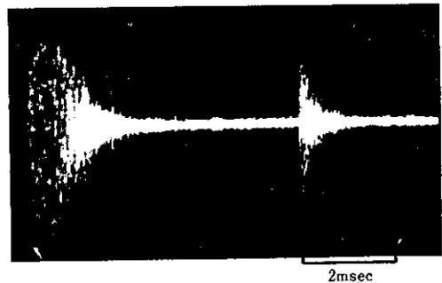
Photo. 1 Example of burst-type acoustic emission observed during deformation of as-quenched 0.3%C steel
