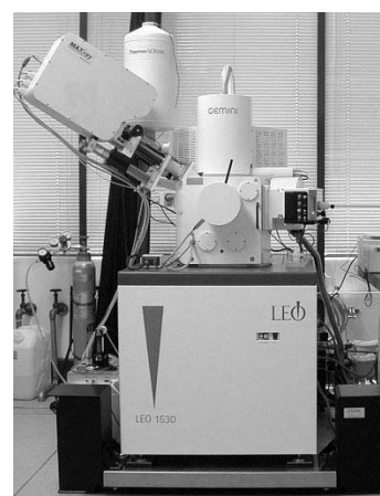
Photo 6 Ultra-low voltage SEM, Gemini
