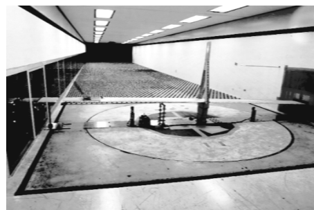
Photo 4 Wind tunnel test for the aerodynamic study on a cable-stayed bridge under construction
