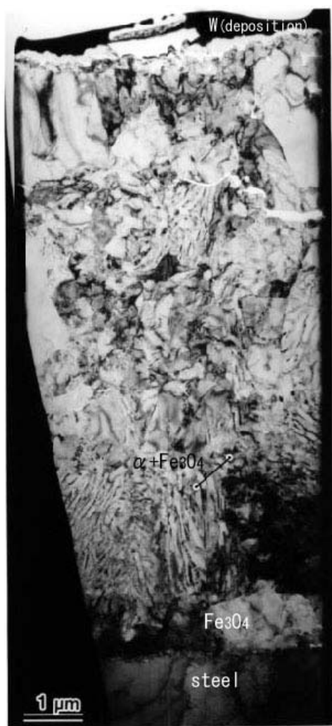
Photo 5 FIB-TEM observation of oxide layer on Al-killed steel
