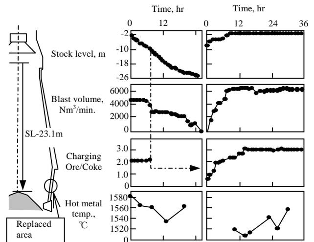
**Fig.3 Operating performance before and after changing Fukuyama No.4 BF's bosh cooling staves**
