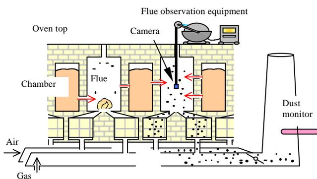
Fig.8 Sensors installed for facilitating efficient oven repair
