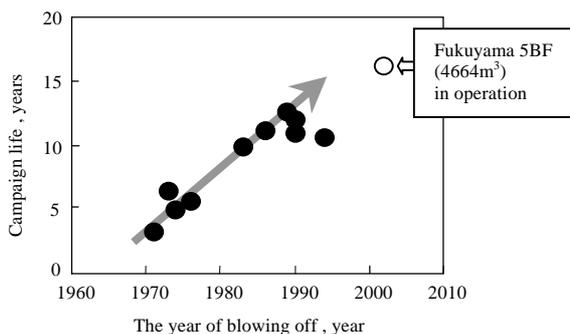
**Fig.2 Transition of NKK's blast furnaces life**
