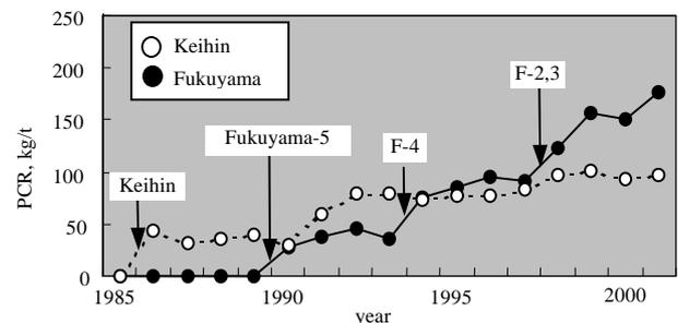
Fig.9 Years of constructing PCI equipment and transition of PCR
