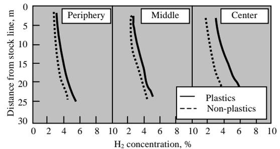
Fig.17 H<sub>2</sub> concentrations in blast furnace top gas during waste plastics injection
