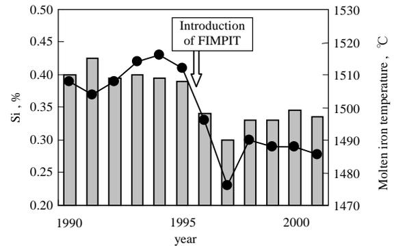
Fig.14 Operational transition before and after the introduction of FIMPIT (Fukuyama)
