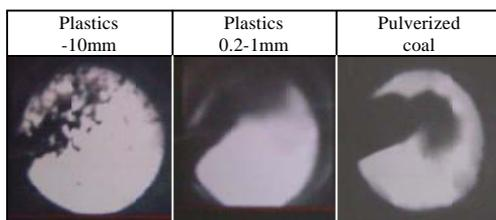
Fig.16 Interior photographs of the tuyere during waste plastics injection
