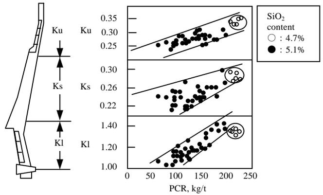
Fig.11 Effects of SiO<sub>2</sub> content in sintered ore on blast furnace permeability
