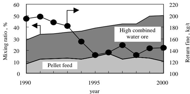
**Fig.4 Transition of material type and return fine rate at NKK's sintering operations**
