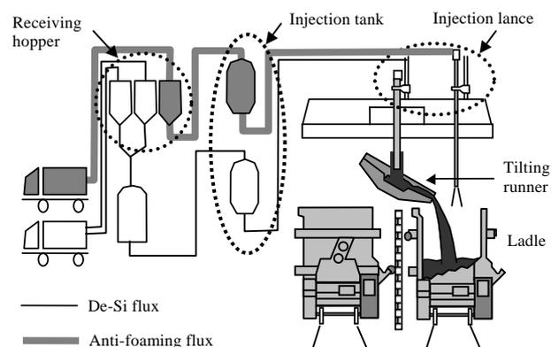
Fig.15 New desiliconization process flow
