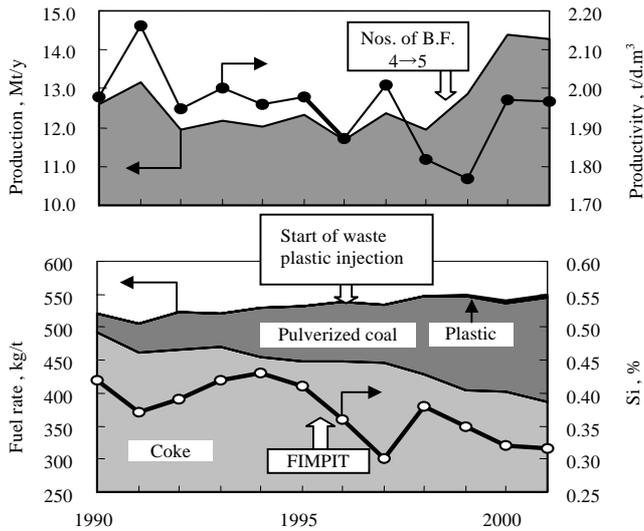
**Fig.1 Transition of major operation parameters within NKK's blast furnaces**
