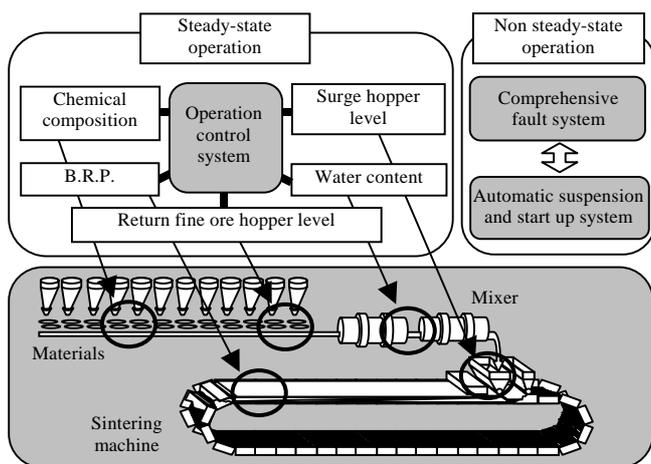
**Fig.5 Operation control systems at the Fukuyama No.4 sintering plant**
