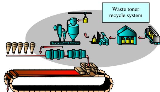
Fig.18 Waste toner recycling system at the Keihin No.1 sintering plant
