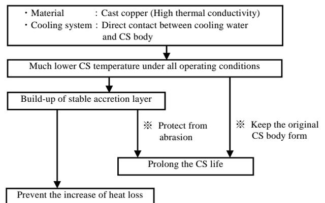
Fig.12 Effect of introducing cast copper cooling staves
