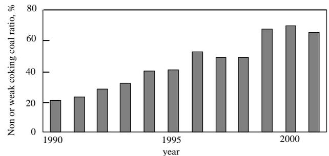
**Fig.6 Transition of non- or weak-coking coal ratio (NKK)**
