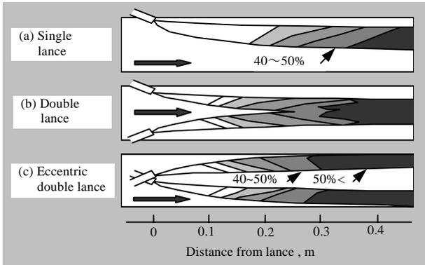
Fig.10 Effects of lance arrangements on pulverized coal flows and combustion efficiency
