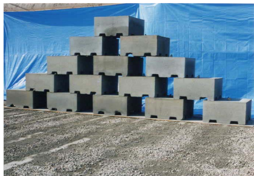
Photo 5 A pile of carbonated slag blocks
