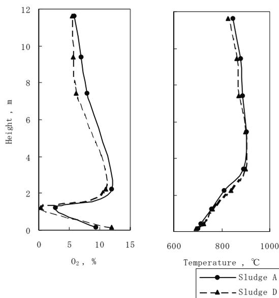
**Fig.5 Profiles of O<sub>2</sub> and temperature in riser**
