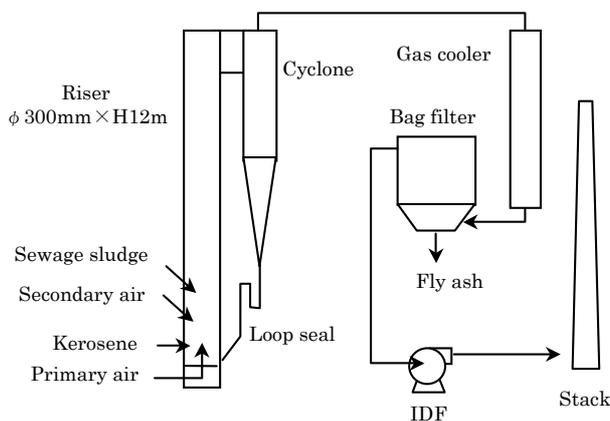
**Fig.1 Pilot plant diagram**
