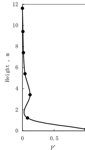
**Fig.2 Pressure profile in riser**
