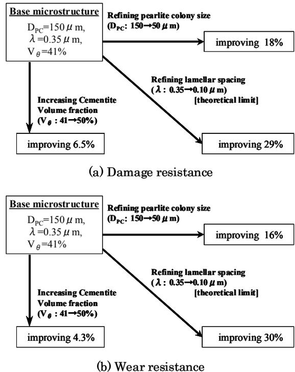
**Fig.4** Improvement of RCF damage and wear resistance through microstructural control
