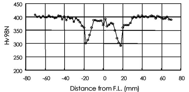
**Fig.10 Hardness distribution near the weld joint**
