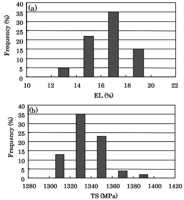
**Fig.5** Production results of the SP rail: (a) EL, (b) TS
