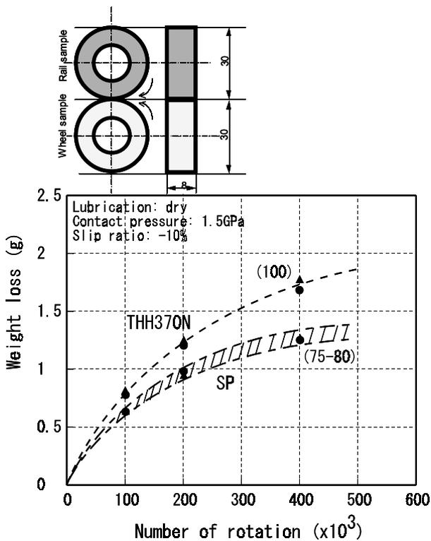
Fig.7 Relationship between weight loss and number of rotations
