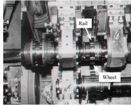
**Photo 1 Appearance of the RCF test machine**
