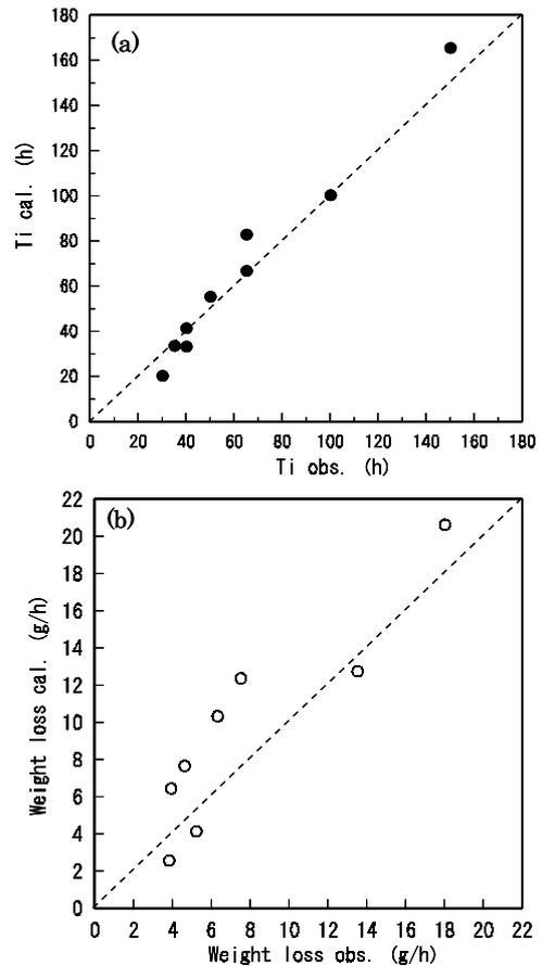
**Fig.3** Observed and calculated values in RCF and wear tests: (a) RCF test, (b) Wear test
