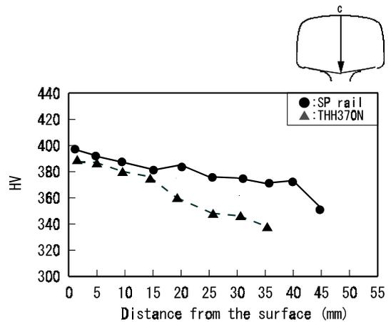
**Fig.6** Hardness distribution from the rail surface
