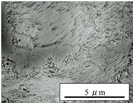
**Photo 4** Microstructure of the SP rail
