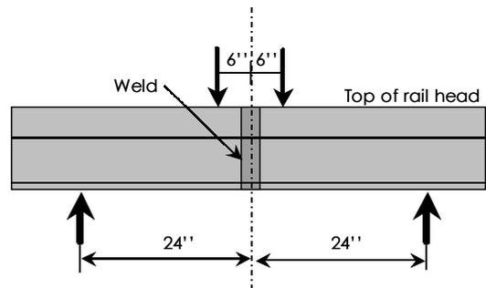
**Fig.11 Test method (4-point bend test)**
