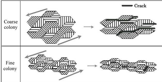
**Fig.8 Improvement of wear resistance through microstructural control (schematic diagram)**
