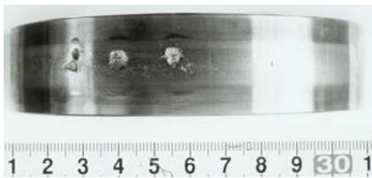
**Photo 3** Appearance of the sample after RCF test
