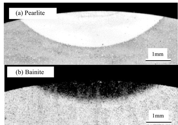
**Photo 5** Macrostructures of samples before flaking test with artificially-made WEL
