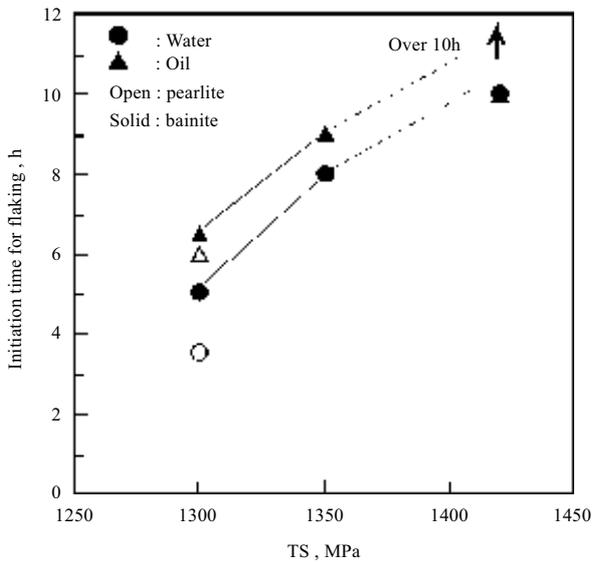
Fig. 2 Flaking resistance in bainitic and pearlitic steels
