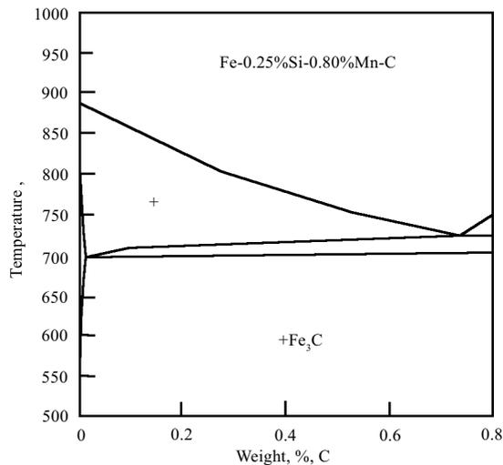
**Fig. 3** Calculated phase diagram for Fe-0.25%Si-0.80%Mn-C system
