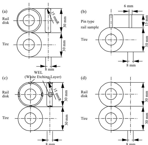
**Fig. 1** Schematics showing of testing configuration;
