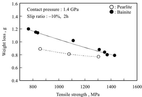
**Fig. 6 Relationship between tensile strength and wear**
