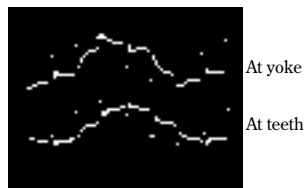
Fig. 7 Differential wave form of flux density in stator core
