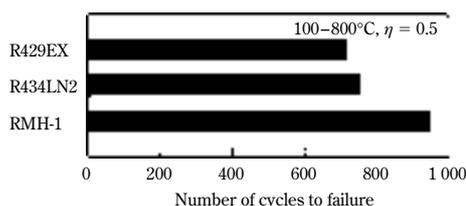
Fig. 7 Comparison of thermal fatigue life between RMH-1 and conventional stainless steels
