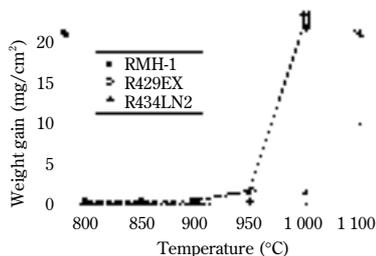
Fig. 5 Oxidation test results of RMH-1, R429EX, and R434LN2 between 800°C and 1 000°C for 400 h in air
