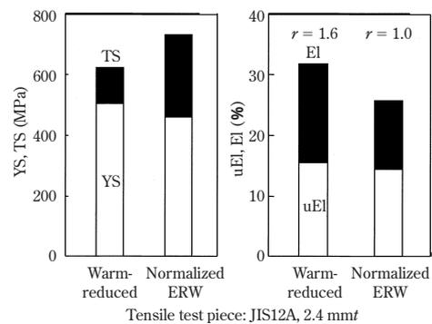
Fig. 2 Tensile properties of warm-reduced high carbon steel tube
