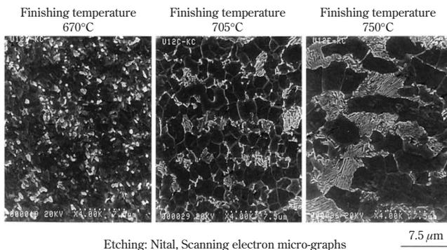
Photo 1 Effect of reducing temperature on microstructure
