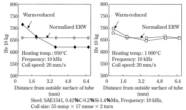
Fig. 6 Effect of heating temperature on induction quenched hardness of warm-reduced steel tube
