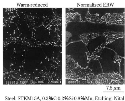
Photo 2 Effect of warm-reducing on microstructure after cold drawing and annealing
