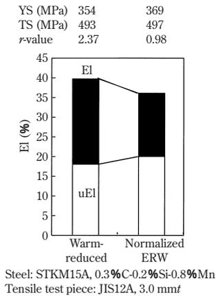
Fig. 5 Effect of warm-reducing on tensile properties after cold drawing and annealing
