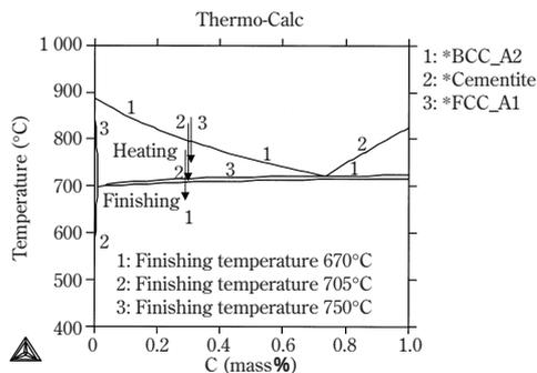
Fig. 1 Reducing temperature and calculated Fe-C-0.2%Si-0.8%Mn phase diagram
