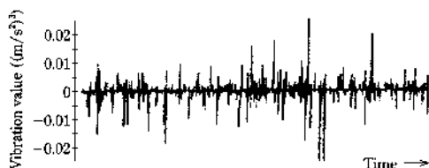
Fig. 4 Treatment wave form of the abnormal bearing
