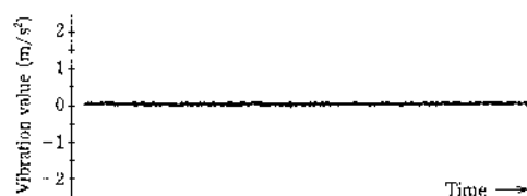
Fig. 1 Original wave form of the normal bearing
