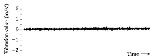
Fig. 2 Original wave form of the abnormal bearing
