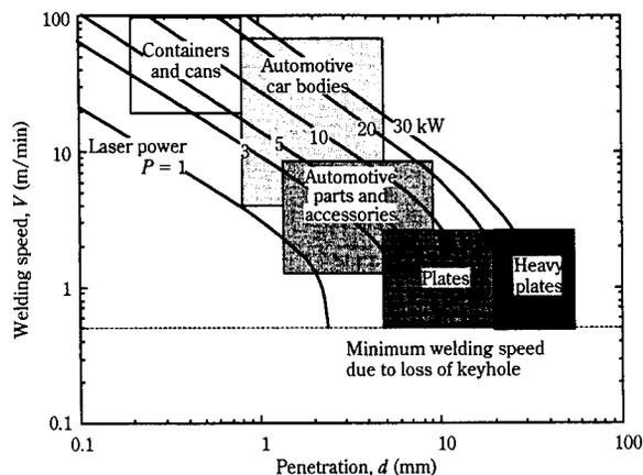
Fig. 10 Relation between laser power and penetration depth of laser welded beads
