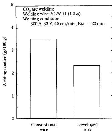
Fig. 1 Comparison between amount of welding spatter in CO<sub>2</sub> arc welding with newly develop wire and that with conventional one
