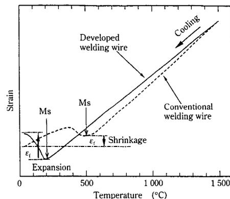
Fig. 2 Change in residual strain of the welding materials after cooling due to the transformation temperature
