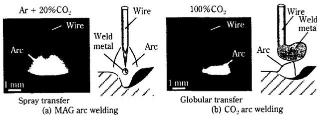
Photo 1 Comparison between MAG (Ar + CO<sub>2</sub>) and CO<sub>2</sub> arc weldings in metal droplet transfer phenomena
