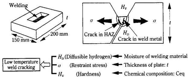
Fig. 6 Factors of low temperature weld cracking
