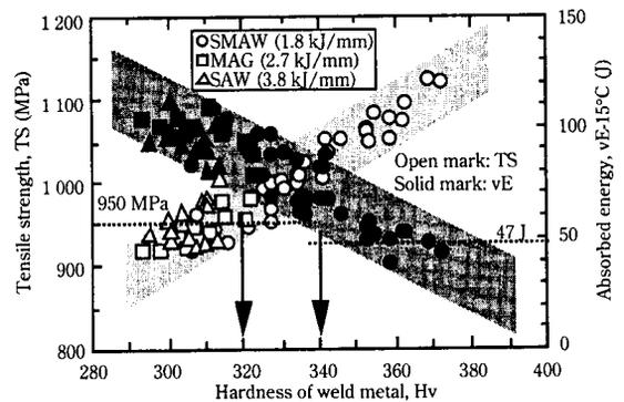
Fig. 7 Relation among hardness, tensile strength and Charpy absorbed energy of the weld metals in the multipass welded joints
