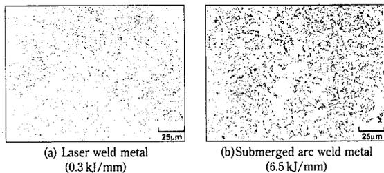
Photo 5 Microstructures of the laser and submerged arc weld metals
