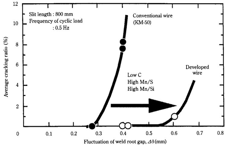
Fig. 5 Relation between fluctuation of root gap and solidification cracking ratio of the weld metal under the cyclic load
