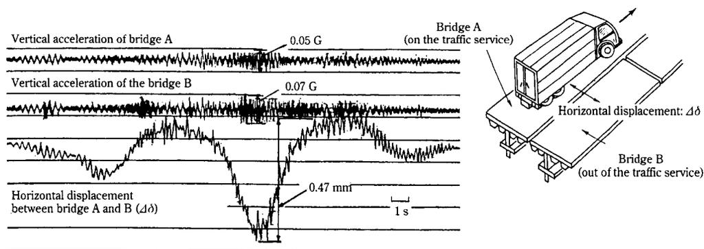
Fig. 4 Example of displacement between bridges on traffic service
