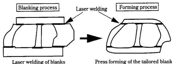
Fig. 9 Example of press forming process with tailored blanking technology
