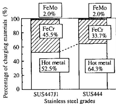
Fig. 12 Comparison of charging materials between SUS447J<sub>1</sub> and SUS444
