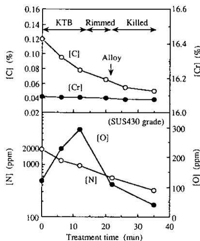
Fig. 7 Change in chemical composition during RH treatment (SUS430 grade)
