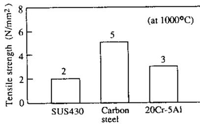
Fig. 16 Comparison of tensile strength at high temperature
