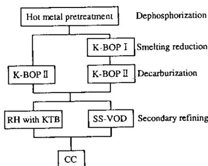
Fig. 1 Process for stainless steelmaking at Chiba Works
