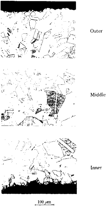
Photo 1 10% oxalic acid etch test results of seamless SUS304 stainless steel pipe
