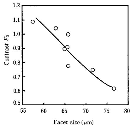
Fig. 4 Relationship between contrast and facet size in HT-80 steels
