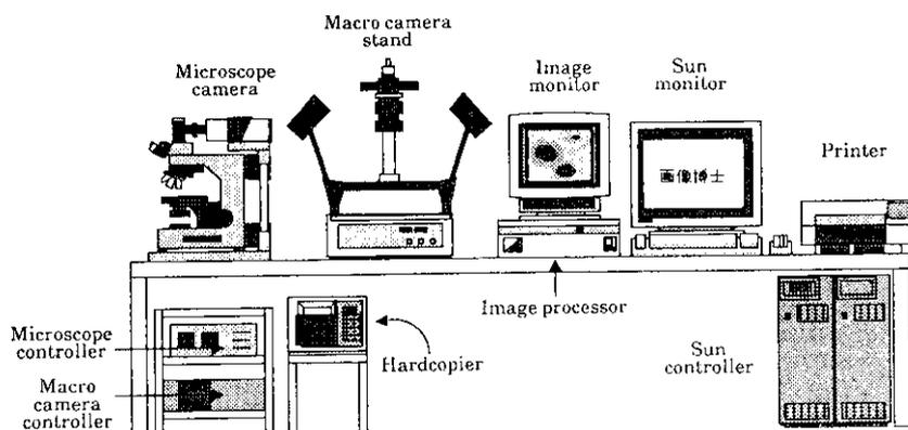
Fig. 6 Standard system configuration of "Dr. Image"
