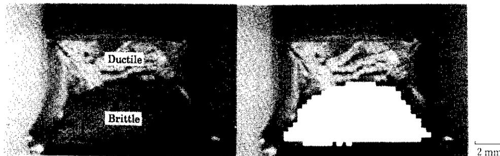
(a) Original image of Charpy fracture appearance (b) Extraction of brittle fracture surfaces
