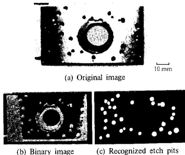
Photo 1 Recognition of etch pits using gray level pattern matching technique
