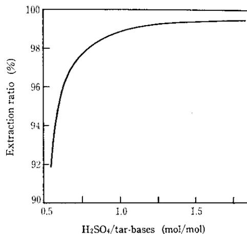
Fig. 2 Effect of sulfuric acid ratio on tar-bases removal
