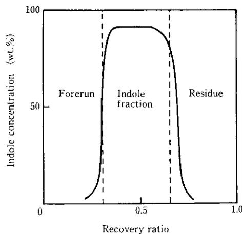
Fig. 3 Distillation curve
