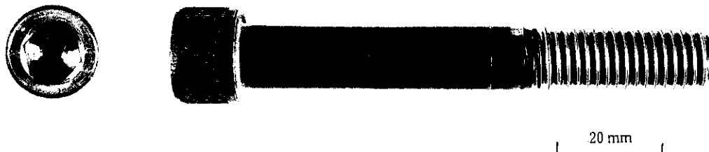
Photo 2 Socket bolt made of direct-softened steel
