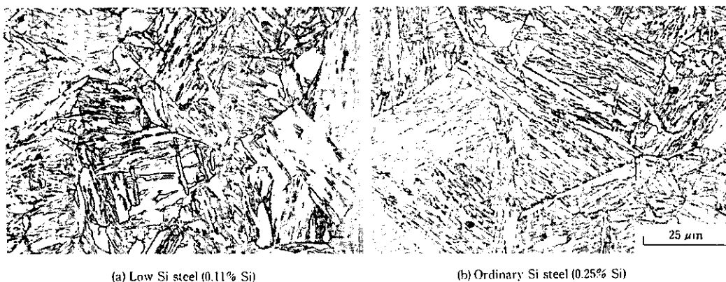
Photo 1 Effect of Si content on martensite structure
