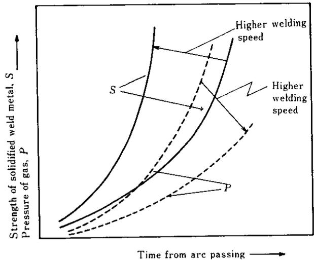
Fig. 9 Change in time curves of solidified weld metal strength and gas pressure by welding speed
