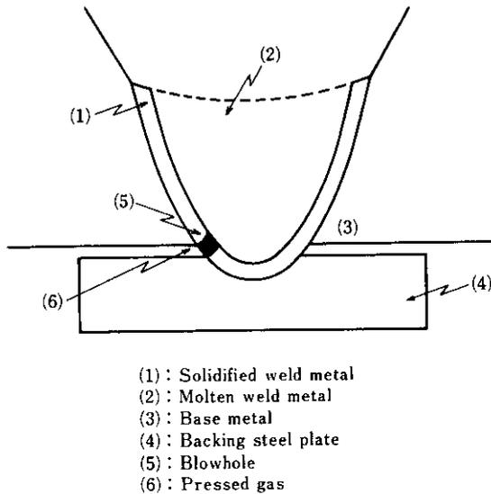
**Fig. 5** Schematic illustration showing occurrence of blowhole
