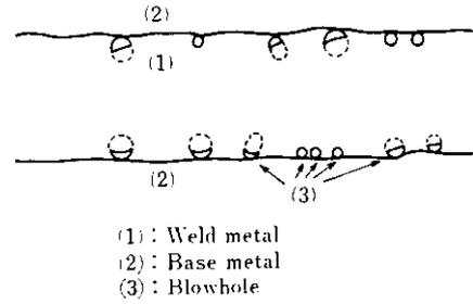
**Photo 6** Horizontal bead section at root showing blowholes occurred
