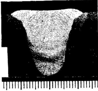
Photo 2 Bead shape of 4° downward welding with V-groove
