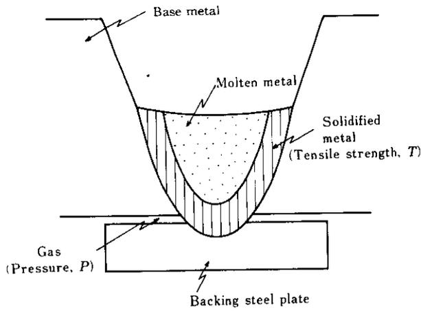
Fig. 7 Schematic illustration showing bead formation
