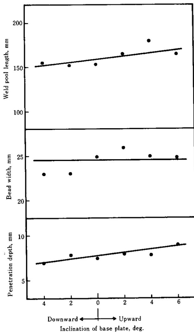
Fig. 3 Change in bead shape and weld pool length by inclination of base plate
