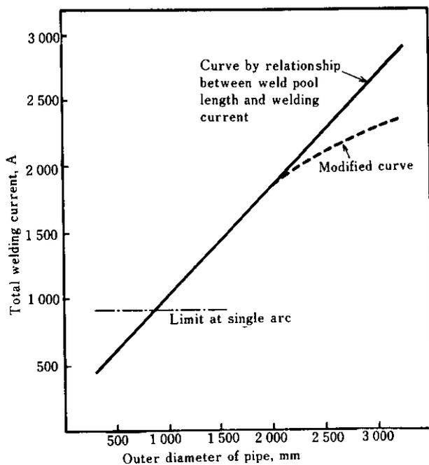
Fig. 4 Available maximum welding current estimation for various outer diameter of pipe
