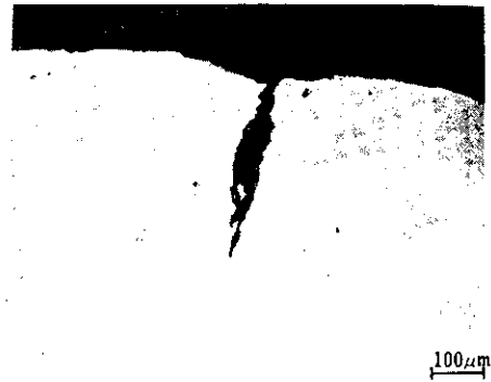
Photo 6 Cross section of penetrator crack
