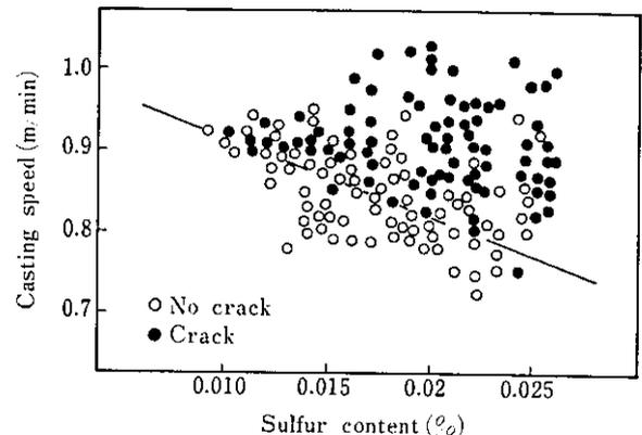
**Fig. 8** Effects of casting speed and sulfur content on internal cracks in web
