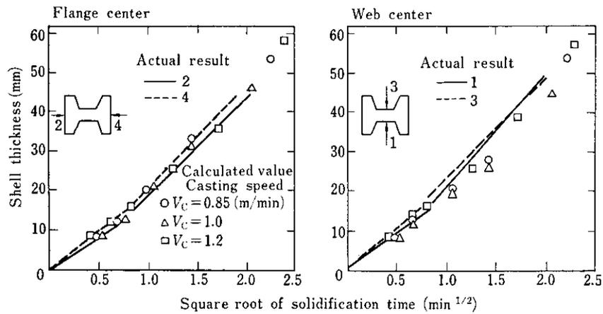
Fig. 11 Comparison of calculated and actual shell thickness
