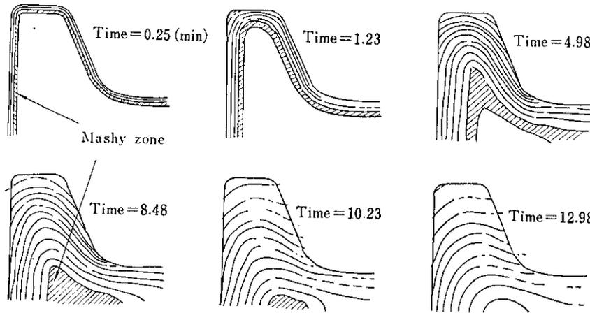
Fig. 12 Progress of solidification of C. C. beam blank by calculation
