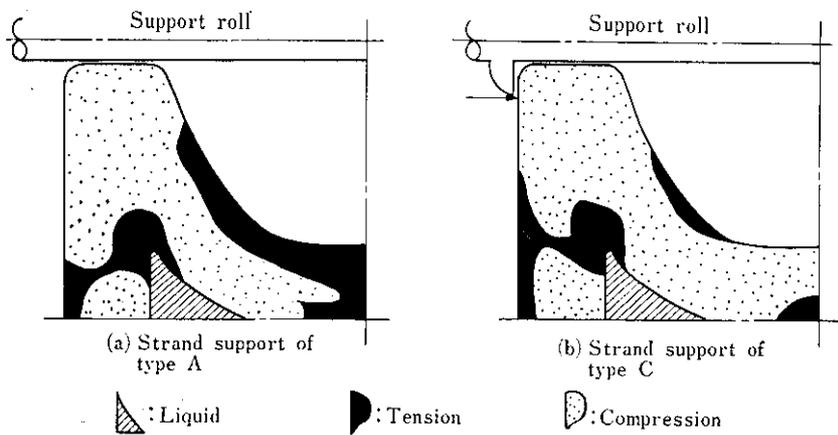
Fig. 17 Stress distribution of beam blank at No. 4 segment
