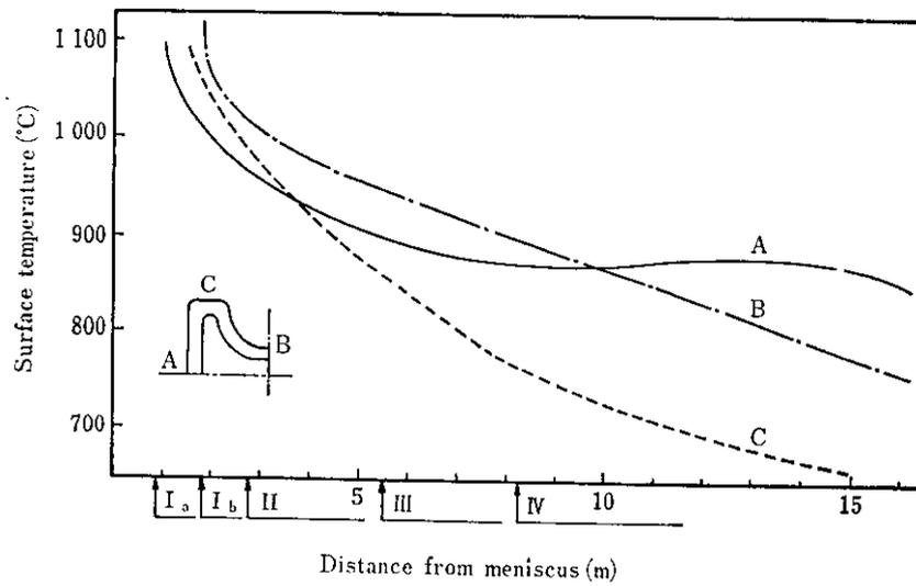
**Fig. 14** Surface temperature of cast steel
