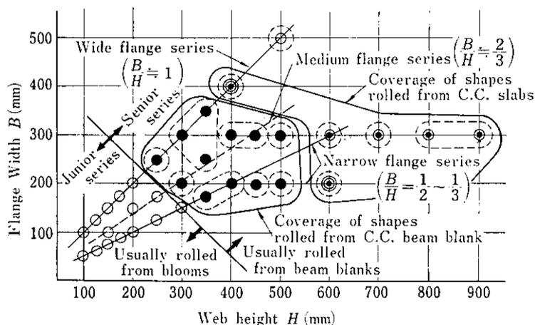
Fig. 21 Relation between wide flange beam sizes and materials
