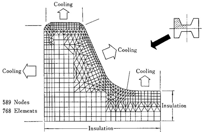
Fig. 9 Modelling for heat transfer analysis
