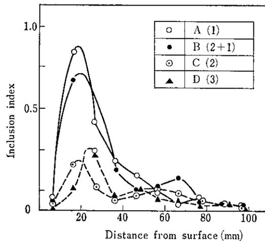
Fig. 6 Effect of the shape of immersed nozzle on the distribution of large inclusions in beam blank casting
