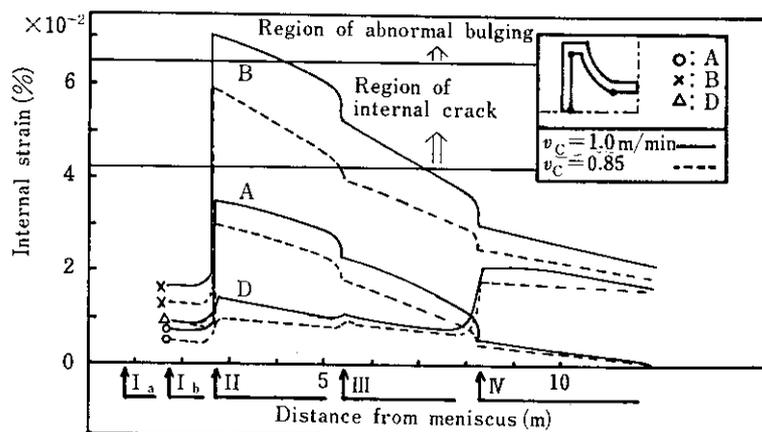
**Fig. 16** Internal strain distribution in strand direction in the case of supporting way of cast blanks shown in Fig. 4
