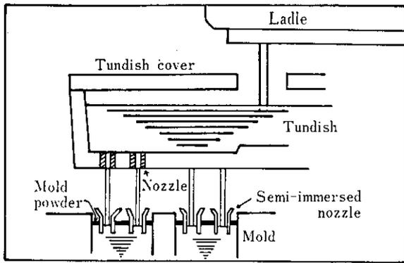
Fig. 5 Schematic representation of casting
