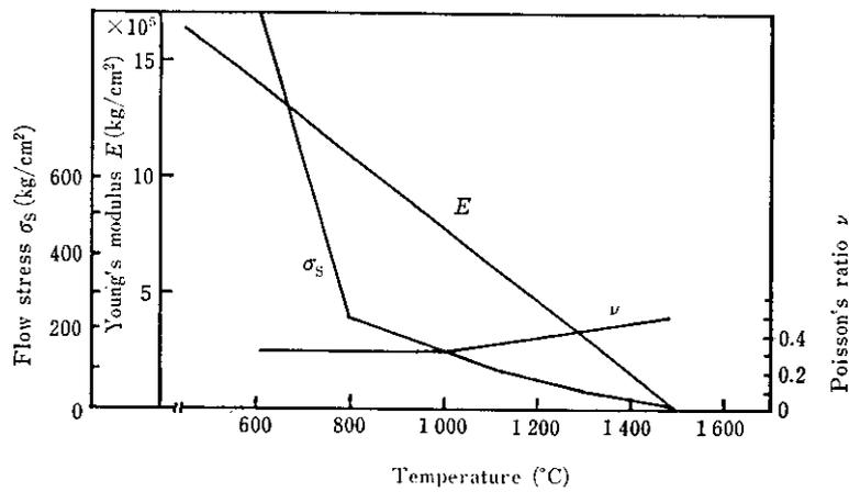
**Fig. 15** Mechanical properties of cast steel
