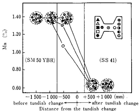
Fig. 20 Change of chemical composition at tundish change
