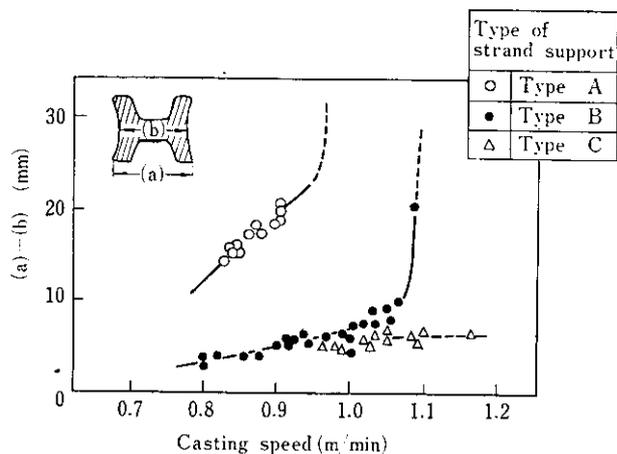
Fig. 19 Relation between casting speed and deformation of B. B.
