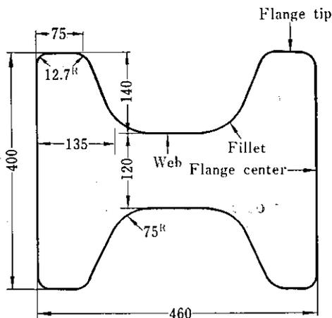
**Fig. 1** Names and size of continuously cast beam blank
