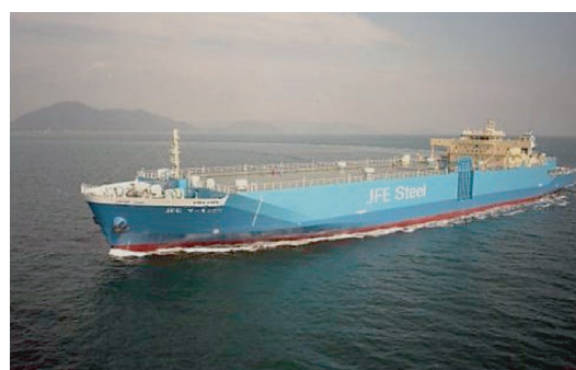
Photo 2 Special ship which can stow cargo pallets in the ship hold by using a mobile loading machine
