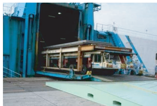
Photo 3 Loading operation for a special ship which can stow cargo pallets in the ship hold by using a special vehicle
