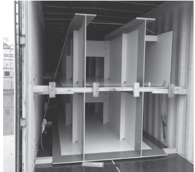
Photo 2 Two-tier stacking of girder blocks in containers
