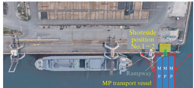
Fig. 9 Monopile transport vessel mooring layout
