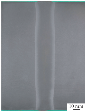
Fig. 3 Photograph in flash-butt welds of SP3 rail
