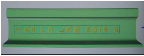
Fig. 5 Example of learned defect (rolled marking on rail)
