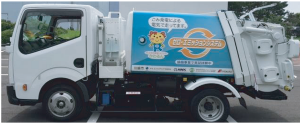
Photo 2 ZeroE waste collecting vehicle with battery cartridge
