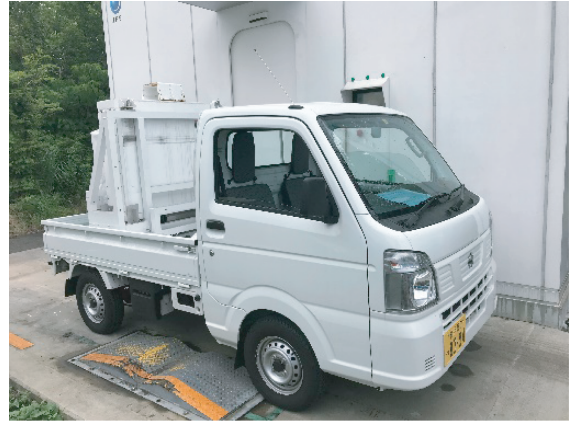
Photo 3 Truck used for battery transport
