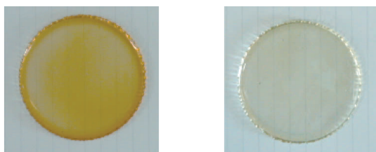
(a) Cured product of alicyclic epoxy resin and dicyclopentadiene type phenolic resin (Light transmittance = 34%) (3.5 mm thickness) (b) Cured product of alicyclic epoxy resin and dicyclopentadiene p -cresol resin (Light transmittance = 76%) (3.5 mm thickness)
