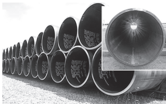
Fig. 7 Appearance of pipes made by NEO press
