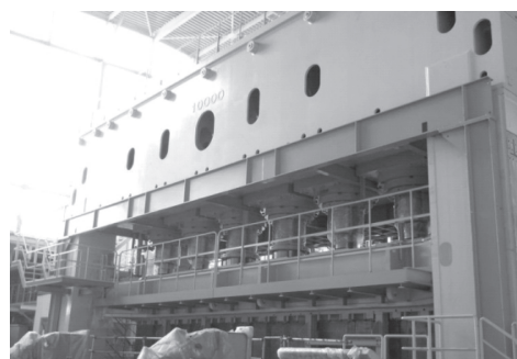
Fig. 5 Press for high productivity press bending (NEO press)
