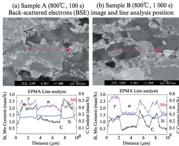
Fig. 4 Field emission-electron probe micro analyzer (FE-EPMA) quantitative line analysis of Si, Mn
