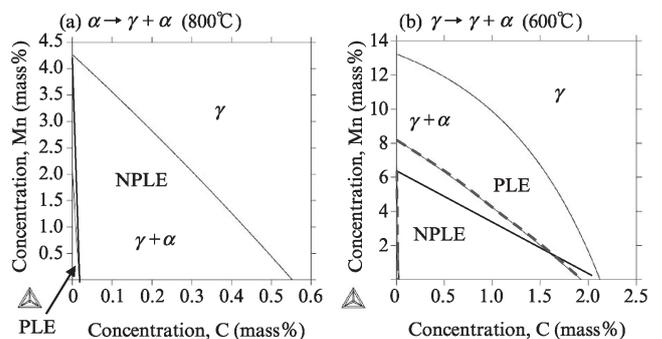
Fig. 7 Calculated isothermal section of Fe-1.4 mass%Si-Mn-C phase diagram at (a) 800°C and (b) 600°C<sup>8)</sup>
