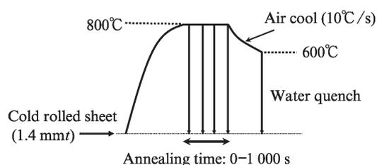
Fig. 1 Schematic diagram of heat treatment<sup>8)</sup>
