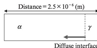
Fig. 3 Geometry models for multi-component diffusion simulation for  $\alpha \rightarrow \gamma$  transformation at isothermal treatment<sup>8)</sup>
