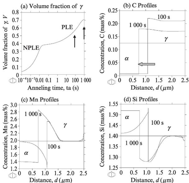
Fig. 5 (a) Calculated variation of the austenite volume fraction with annealing time and (b) C, (c) Mn, (d) Si profiles in 100 s, 1000 s during 800°C holding<sup>8)</sup>
