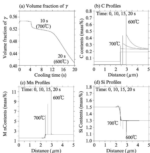
Fig. 8 (a) Calculated variation of the austenite volume fraction with cooling time from 800°C, 100 s and (b) C, (c) Mn, (d) Si profiles<sup>8)</sup>
