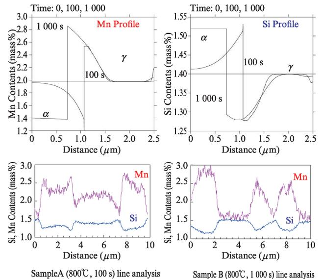
Fig. 6 Comparison between DICTRA Si, Mn profiles and field emission-electron probe micro analyzer (FE-EPMA) line analysis
