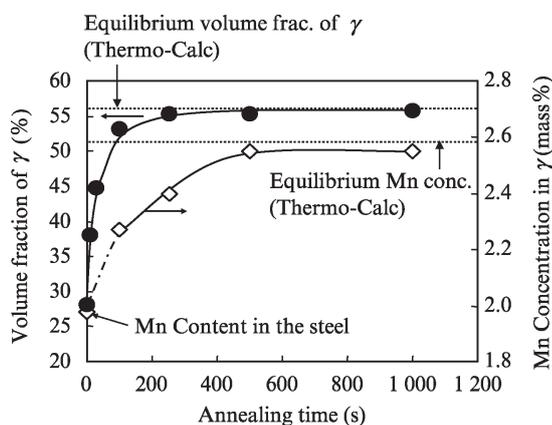
Fig. 2 Variation of the austenite volume fraction and Mn concentration in  $\gamma$  with annealing time at 800°C<sup>8)</sup>
