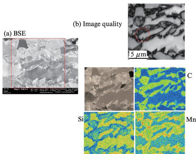
Fig. 9 (a) Back-scattered electrons (BSE) image, (b) Image quality of electron back-scattering pattern (EBSP) and (c) Field emission-electron probe micro analyzer (FE-EPMA) C, Mn, Si mapping on same position of sample C<sup>8)</sup>
