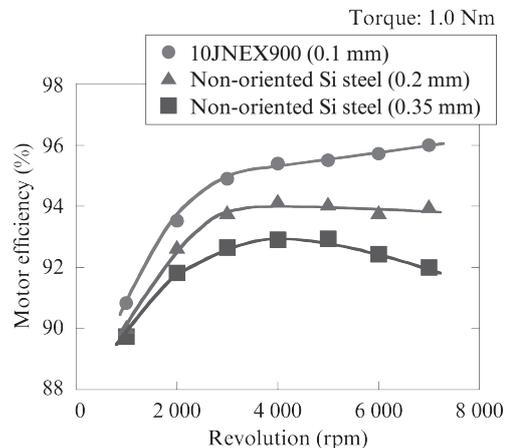
Fig. 7 Motor efficiency and motor speed<sup>4)</sup>
