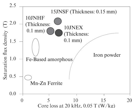
Fig. 3 Overview of magnetic property at high frequency
