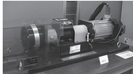
Photo 3 Model motor evaluation system
