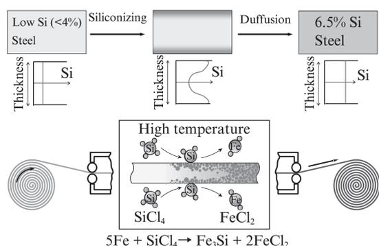
Fig. 1 Manufacturing process of 6.5% Si steel
