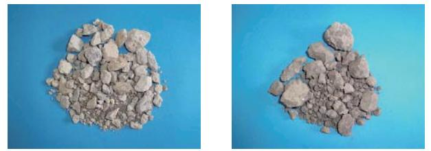
(3) No. 3 Air-cooled blast furnace slag
