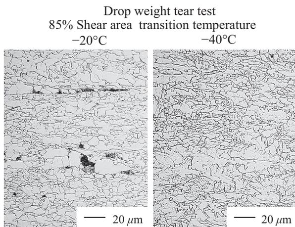
Photo 1 Influence of microstructure on toughness (API X70 electric resistance welded linepipe)
