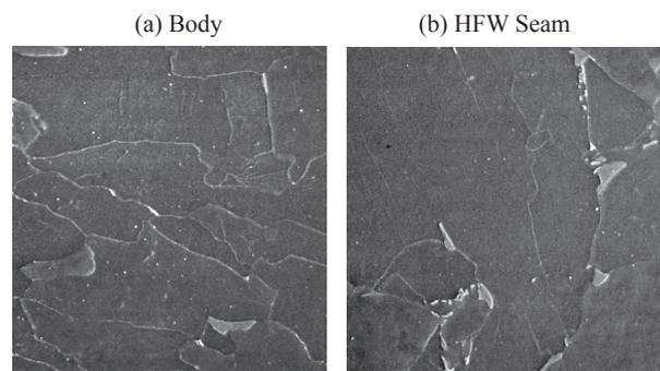
Photo 3 Microstructure of electric resistance welded pipe
