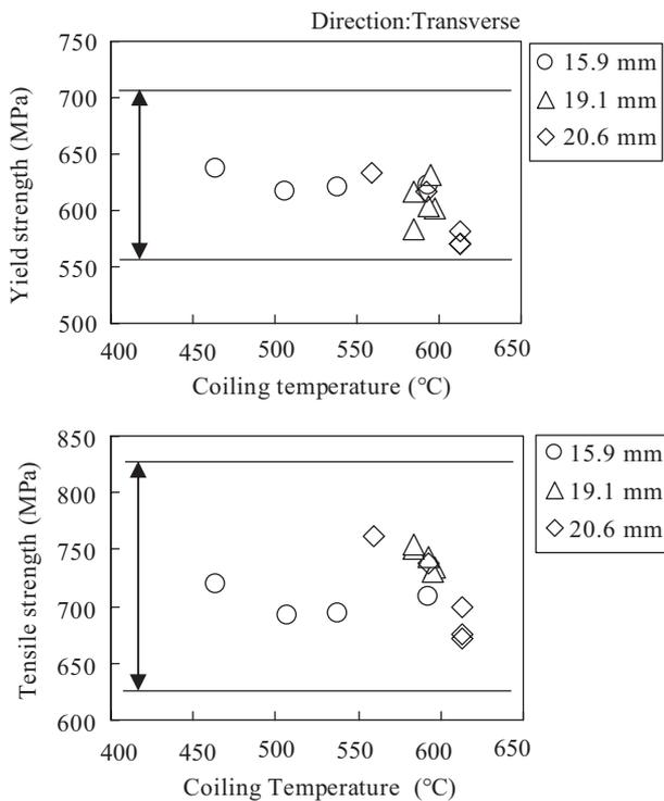
Fig. 6 Tensile properties of API X80 pipes
