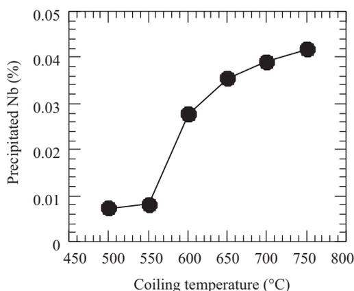
Fig. 5 Relation between precipitated Nb amount and coiling temperature (0.05% Nb steel)
