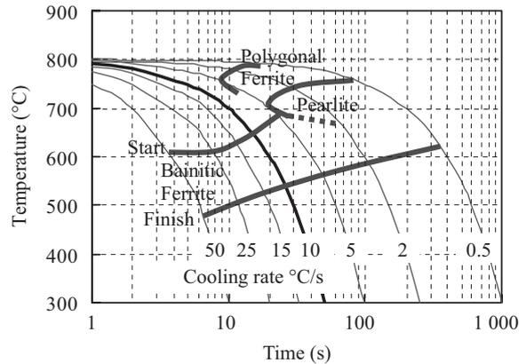
Fig. 3 Continuous cooling transformation diagram of steel B
