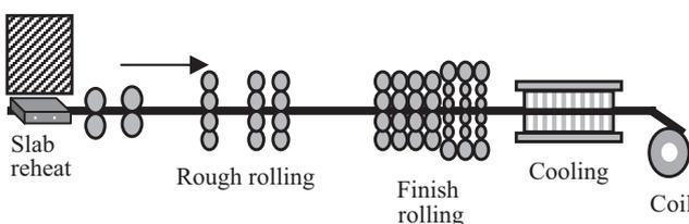
Fig. 1 Hot rolling process
