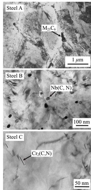
Photo 1 TEM images of precipitates in Steel A(base), B(Nb added), and C(high N) tempered at 550°C for 60 min
