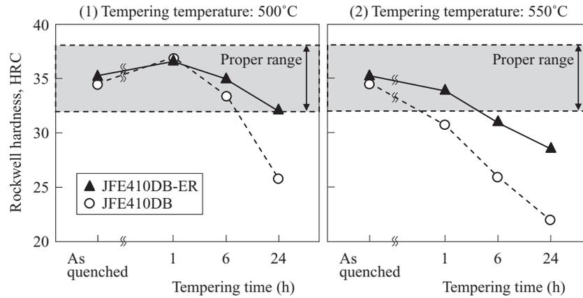
Fig. 9 Change in hardness with tempering time at (1) 500°C, (2) 550°C in JFE410DB-ER and JFE410DB
