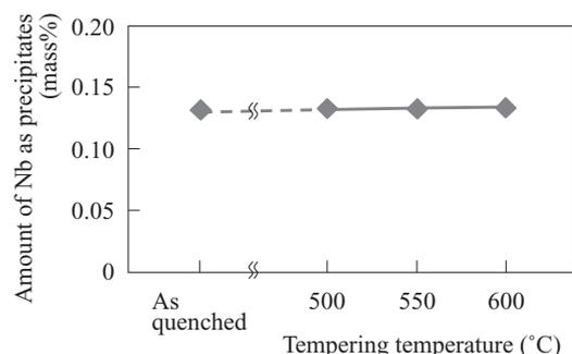
Fig. 5 Amount of Nb as precipitates in Steel B(Nb added) tempered at each temperature for 60 min.
