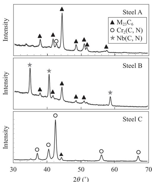
Fig. 4 X-ray diffraction intensity of precipitates in Steel A (base), B(Nb added), and C(high N) tempered at 550°C
