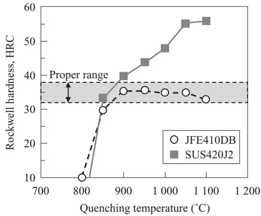
Fig. 2 Quenching hardenability in JFE410DB and SUS420J2 (Specimens were quenched by air cooling after holding at each temperature for 10 min.)
