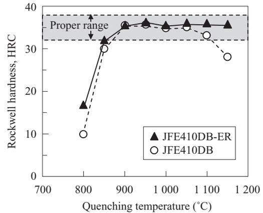
Fig. 7 Change in hardness with quenching temperature in JFE410DB-ER and JFE410DB
