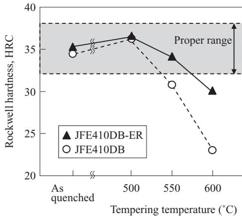
Fig. 8 Change in hardness with tempering temperature in JFE410DB-ER and JFE410DB
