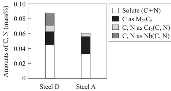
Fig. 6 Amount of solute/precipitated C, N in Steel A(base), and D(Nb + high N) tempered at 550°C
